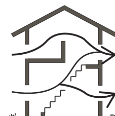
Strategically locating doors & windows during the design phase of your home can promote good conditions for cross-ventilation
